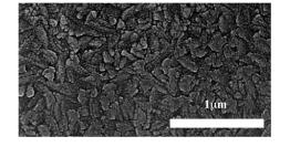
**Supplementary Fig. 2** SEM image of the surface of the ITO electrode immersed in the aqueous solution containing SWNTs•SDS complex.
